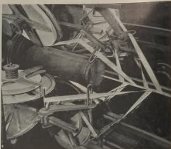
Perfect registration of the layers of insulating paper is an essential feature of the paper-lapping process
