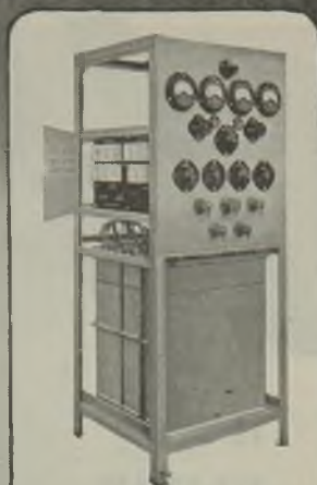
A Multi-Circuit Rectifier Cubicle, having Metal Rectifiers and Transformers, housed in Vapour-Tight Oil-Filled Tanks for working in a very corrosive atmosphere.
