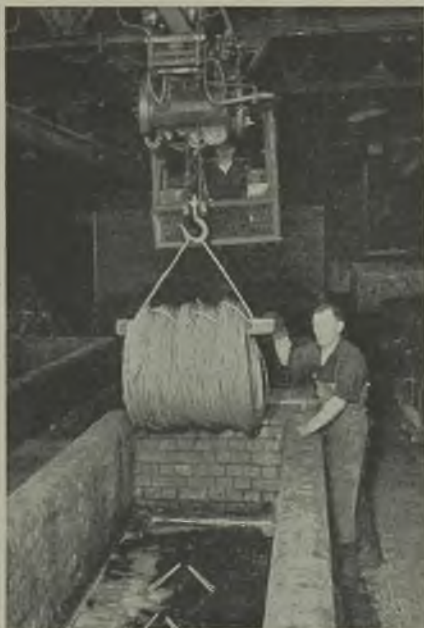
The coils of copper rod are first "pickled" in a dilute solution of sulphuric acid; lifting operation
