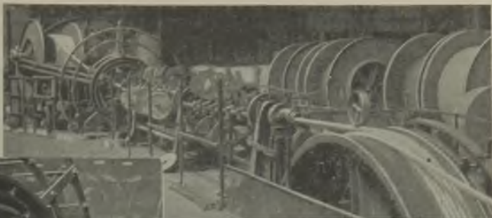
The carriages are rotated at suitable speeds conforming to the lay of the cores as these are passed through the die plate
