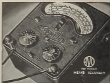
The 50-range Model 7 Universal AvoMeter.
