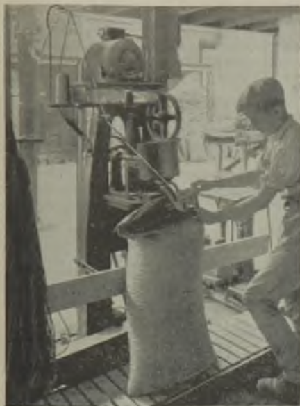
The sacks are closed by means of an electric stitching machine
