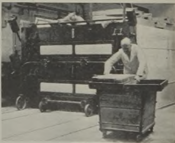
Large electric bakers' oven in use at Carrick's bakery
