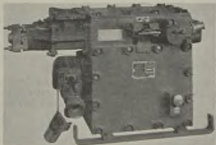
Contactor room-switch for coal-face machines
