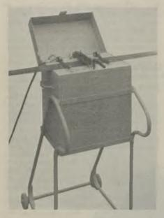
Fig. 2.-Seam welder for plastic strip and sheet
