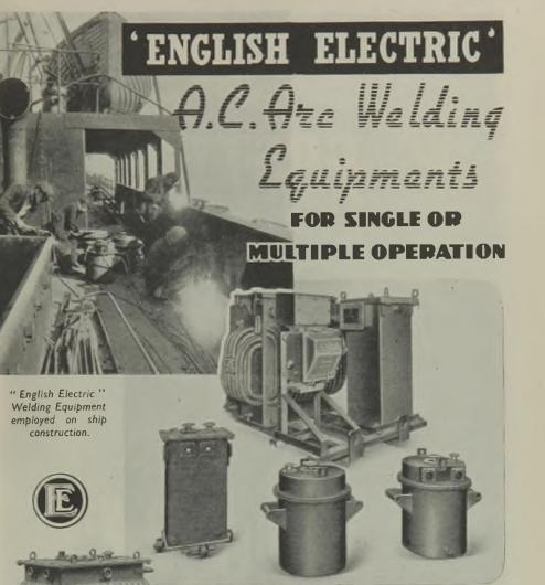
The above illustration shows a transportable multi-operator welding transformer equipment, comprising 3-phase welding transformer with primary and secondary protected type terminals, primary triple-pole "English Electric" fuse-switch and power factor improvement condenser, with two 300-amp. and one 600-amp. welding regulators.
