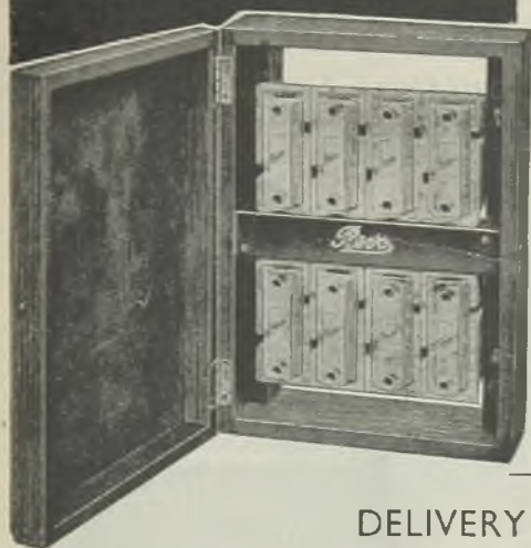
Revo S.3420. Teak Cased Fuseboard. Available for 15 Amp 500 V, 30 Amp 250 V, 30 Amp 500V, 40 Amp 250 V, for 2-10 ways.
