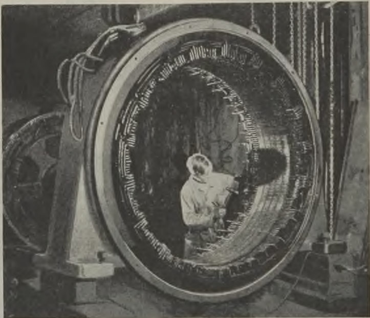
STATOR OF AUTO-SYNCHRONOUS MOTOR REWOUND AT OUR WORKS
