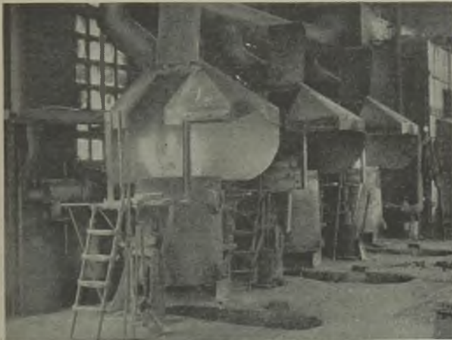
Three 400-lb. Morgan tilting furnaces and three of a line of seven pit fires (right) are connected to the pipe-line of the non-ferrous foundry installation; note pre-heaters
