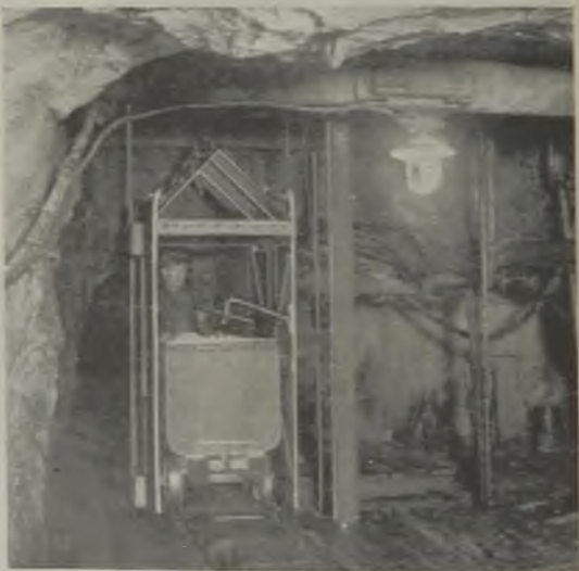
The cars are hoisted up the twin-cage shaft by a surface winder; shaft bottom
