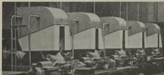
Grinding machine fitted with oil-spray filter
