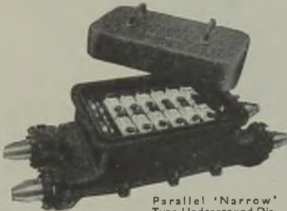
Parallel 'Narrow' Type Underground Disconnecting Box with Bolt on Wiping Glands. The fuses are provided with Porcelain Carriers which can be fitted instead of the Bakelite Lifting Bars supplied as standard.
