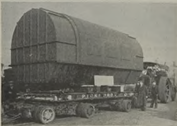
English Electric 125-ton stator on its way to Blackburn
