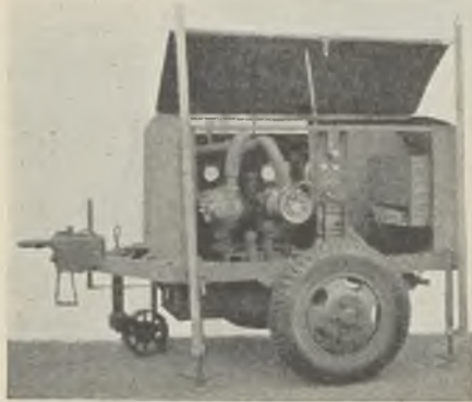
Generator test set (12-kW) with one "Type P" and one American 6-kW generators.
