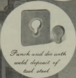
Mild steel punch and die after machining.
