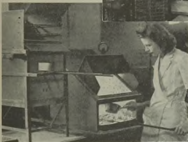
Above: Sifting vitreous enamelling powder on to resistances during treatment in electric furnaces Right: Winding a 100-ohm resistance with 0.001-in. wire, the resistance being measured during winding by the instrument on the left
