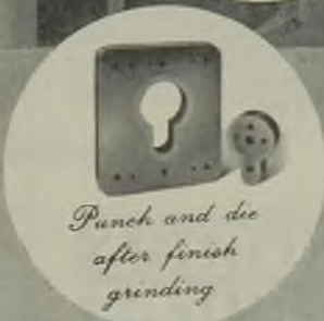
Punch and die with weld deposit of tool steel.
