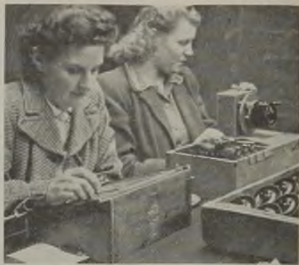
Checking the linearity of scanner potentiometers for radar work
