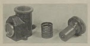
Combined magnetic oil filter and flow indicator
