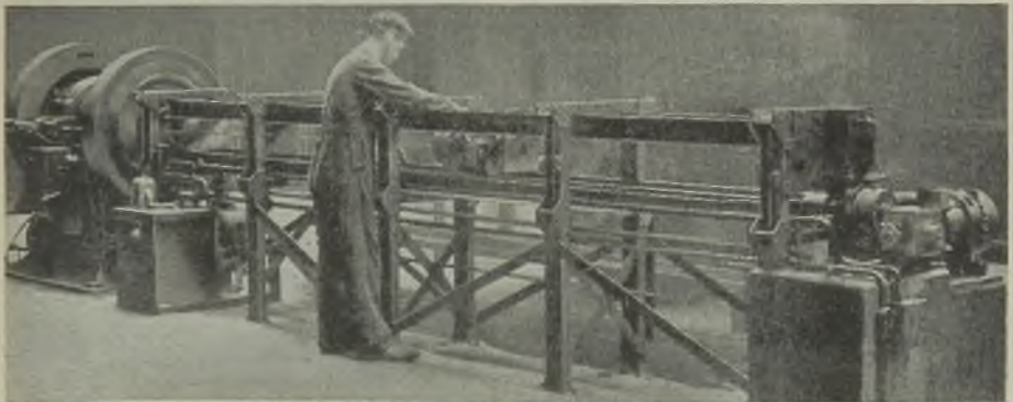
Intermittent swaging machine for waisting a number of portions on a 10-ft. bar
