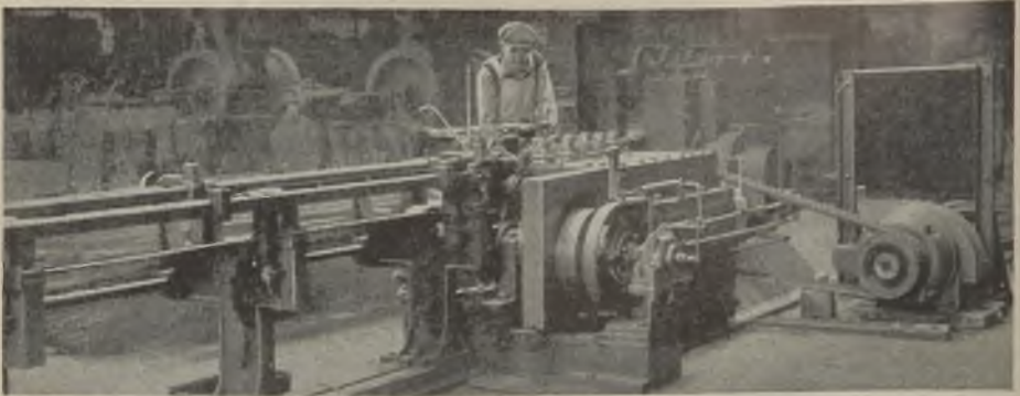
Rod under treatment in this straightening machine passes through flying shears
