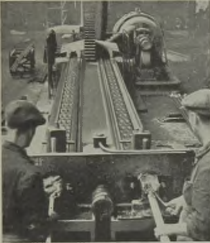
Above: The driving motor for this draw bench was originally a totally-enclosed motor, but has since been modified for pipe ventilation. Right: Drawing machine, driven by an AC commutator motor, which requires a widely varying speed on starting up
