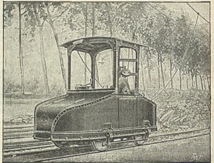
Abb. 111. Treidellokomotive System Chanay, 1904
