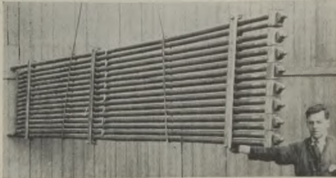
Section assembly of the steel-tube flash-welded economiser
