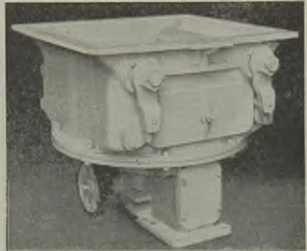
Feeders on the storage bins pass the pulverised coal into the air stream serving the four tangential burners
