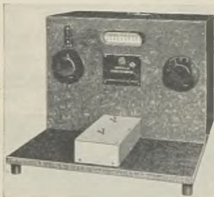
"Metroflux" magnetic sorter for checking small iron bolts against a standard
