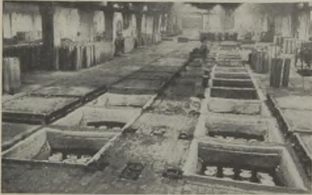
Firing is effected on the continuous-firing principle in ring-type producer-gas furnaces
