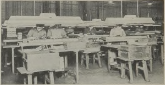
Final inspection and boxing are carried out on benches served by specially disposed fluorescent lighting fittings
