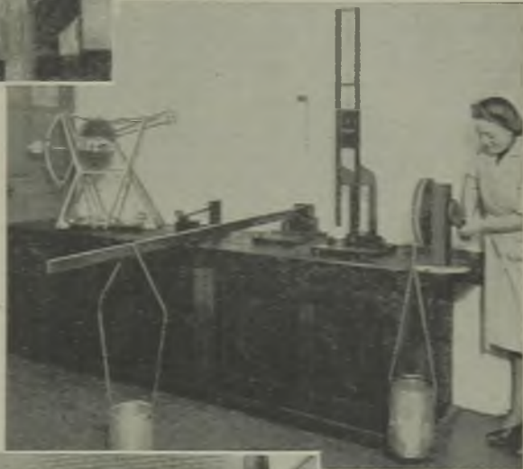
Above: The load on the E.R.A. impact machine (left-hand of picture) can be varied from 1/2 ft.-lb. up to 13 ft.-lb.; mechanical testing includes torque tests (right-hand) and blow and transverse testing for telephone cradles and handles. Left: A feature of the chemical laboratory is the absence of bench sinks, water being available at any point, and waste removed by continuous water channels
