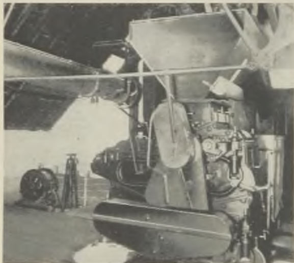
A 15-HP motor belt drives the grist mill
