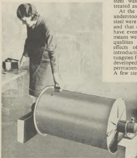
Fig. 1.—Magnetic separator drum, 30 in. by 20 in. diameter, giving performance equivalent to that of an electro-magnetic drum of the same size
