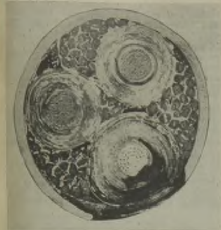
Fig. 7.—Section of three-core 0.15 sq. in. 33-kV cable at point of breakdown
