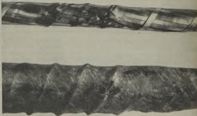
Fig. 6.—Subsidiary fault, showing rib markings on lead sheath and B.o.T. tapes with small burst
