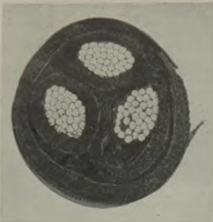
Fig. 3.—Section of cable showing cracked belt and loose core insulation
