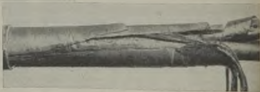
Fig. 2.—Belt insulation cracked along the lay of the cores
