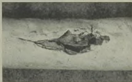
Fig. 4.—Burn-out in lead sheath on 0.05 sq. in. cable
