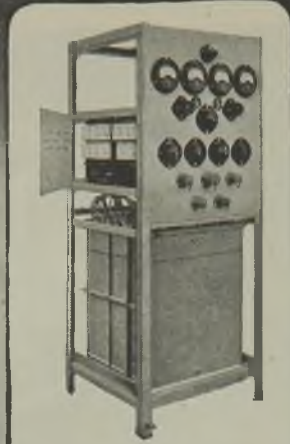
A Multi-Circuit Rectifier Cubicle, having Metal Rectifiers and Transformers, housed in Vapour-Tight Oil-Filled Tanks for working in a very corrosive atmosphere.
