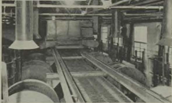
Above: Each cracking mill is driven by a 150-HP pipe-ventilated motor; all the starting equipment for this motor is housed in an iron-clad cabinet with hinged doors Right: A motor-driven travelling hopper (above) discharges the mixture into steam-heated revolving spherical digestors below
