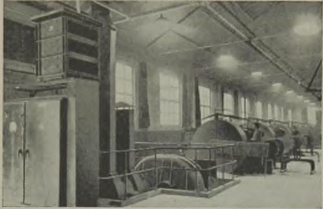
The refining machines are group driven by a 275-HP motor for each battery of three machines
