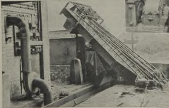
A new development in grass drying for winter fodder which is believed to represent a considerable advance on the rotary type of dryer. Above: Furnace housing and dryer showing conveyor-drives. Below: Elevator to the dryer and dried grass cooling fan. Right: Chaff cutter, grinder and fan fed by conveyor from the drying cabinet
