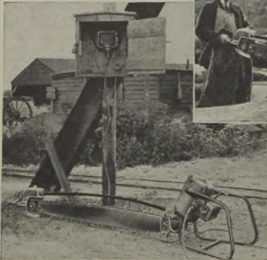
There is a continuous call for timber on the farm, so that a big aid is the portable cross-cut saw; supply unit is seen in pole-mounted cupboard
