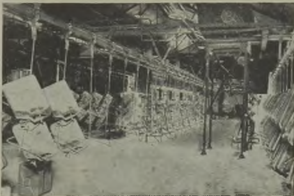
One of ten ferric paint drying installations 502 kW using 2008 Osram Infra-Red Industrial Lamps
