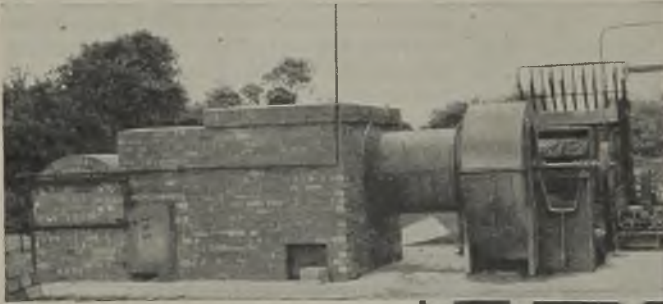
A new development in grass drying for winter fodder which is believed to represent a considerable advance on the rotary type of dryer. Above: Furnace housing and dryer showing conveyor-drives. Below: Elevator to the dryer and dried grass cooling fan. Right: Chaff cutter, grinder and fan fed by conveyor from the drying cabinet
