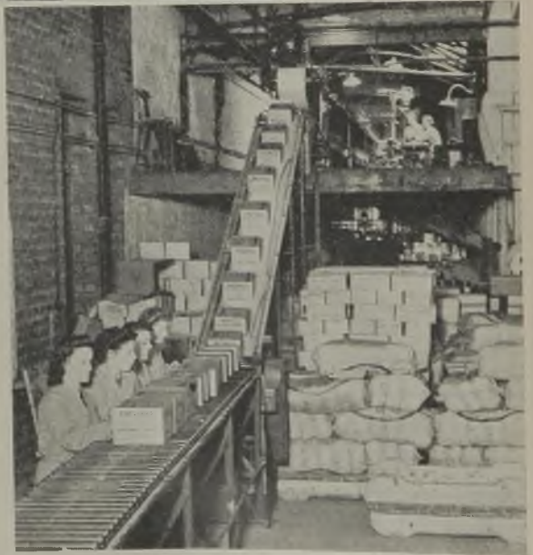
Right: A 1-HP motor driven inclined conveyor passes the cartons from the compressor conveyor to an idle roller conveyor in the packing department
