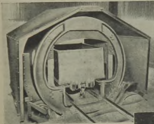
Above : From the weighing machine the tubs are passed on to any of three revolving tipplers, according to the class of coal they contain Right : The vacuum flotation machine is so constructed that any normal variation in the rate of flow is automatically compensated for by the opening and closing of a float control valve
