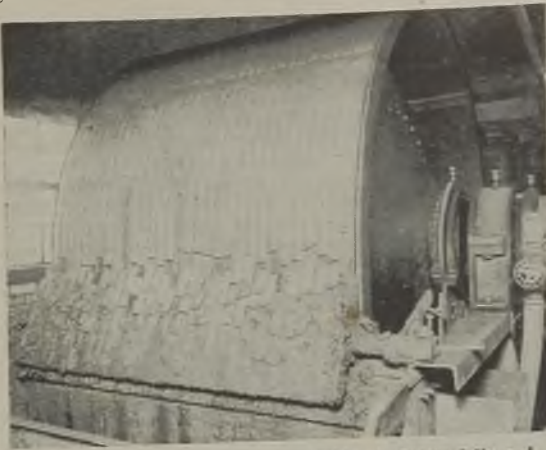
The production of the flotation machine is finally delivered, still as slurry, to the trough of a vacuum drum type filter; "cake" for mixing with the washed slack is removed from the rotating drum
