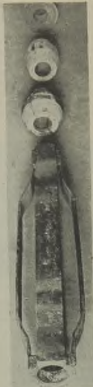
Spring-steel contactor unit and wood insulators on the production pipe; a special moulded top insulator at the top carries the weight of the pipe
