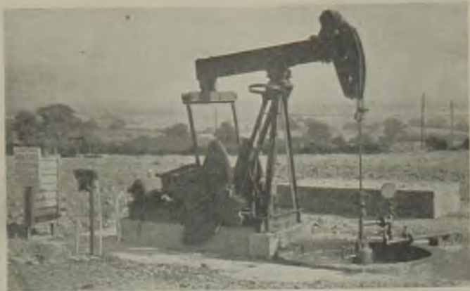
All the well motors (above) are of the beam type, rather like Cornish pumps. Left: Mud is pumped down the drill pipe by a 150-HP motor driven pump; drilling motor at rear right
