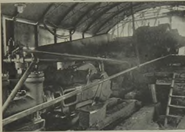
All the well motors (above) are of the beam type, rather like Cornish pumps. Left: Mud is pumped down the drill pipe by a 150-HP motor driven pump; drilling motor at rear right
