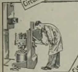
Circuit Breaker Truck withdrawn from cubicle
