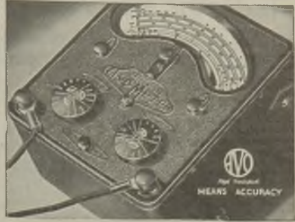
The 50-range Model 7 Universal AvoMeter.
