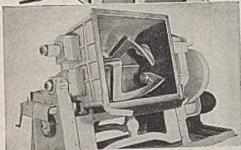
Mixer used in the preparation of a sizing clay solution for the loading of magazine paper stock. It was fabricated of 20% Lukens Nickel-Clad Steel by the J. H. Day Co., Cincinnati, Ohio.
