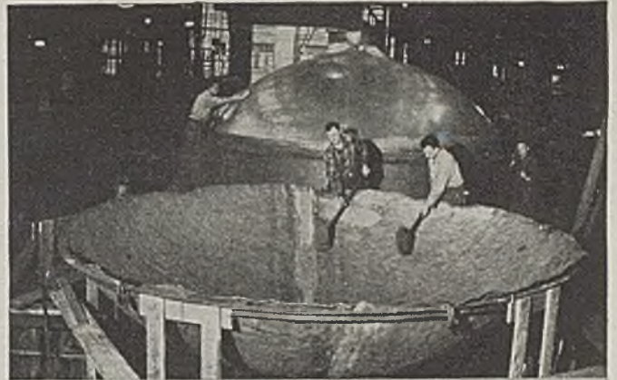
Rough-forming copper dome of a 16' kettle
