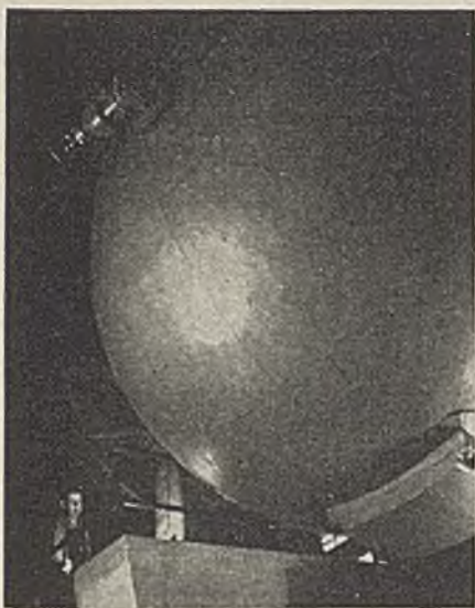
In spherical, revolving digesters the fiber is treated with chemicals
