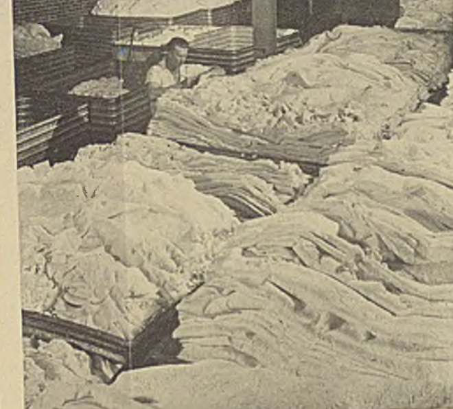
3 In the paper mill stock is stored in shredded lap form in galvanized iron boxes which can be easily handled by electric lift trucks or other means
