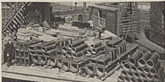
RUBBER-LINED EQUIPMENT FOR METAL PICKLING PLANT —Spent liquor sewers, fume exhaust ducts and stacks, drain piping and fittings all lined with Manhattan Acid-Proof Rubber Lining. For use in continuous strip pickling process in large steel mill. This part-shipment weighed 15 tons.
