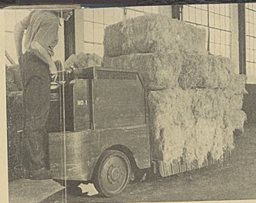
1 Decorticated flax straw in 150 to 160-lb. bales is conveyed from box cars to storage in large warehouses having a floor space of five acres, or directly to the pulp mill. A year's requirements must be kept on hand
