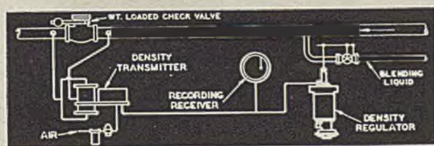
Typical installation for measurement and regulation of density
