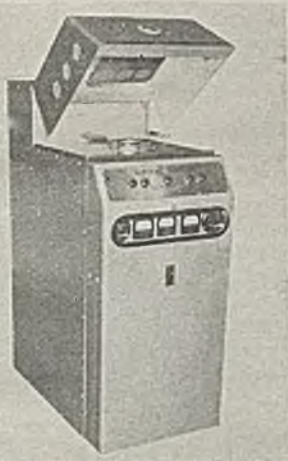
5-kw. preform preheater
