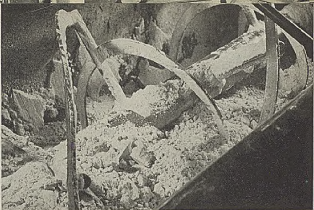
Batch of dry components is transferred into blender and resin and plasticizers added. Latter is sprayed over mass for best mixing results
