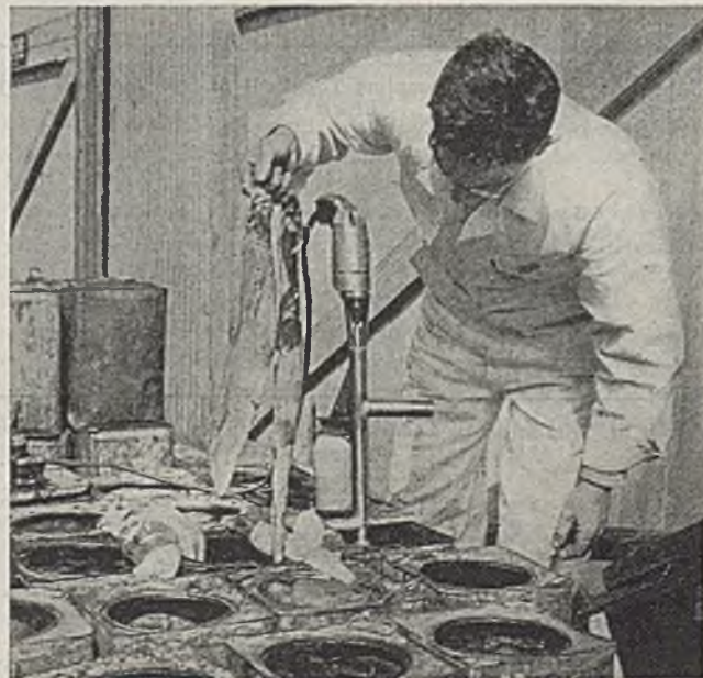
Figure 2. Motor-Driven Core Sampler in Use Some shark livers are exposed to show nature of material
