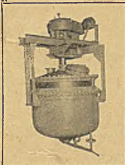
Large Steam jacketed copper boiling and mixing pan with geared agitators, steam jacket of mild steel.
