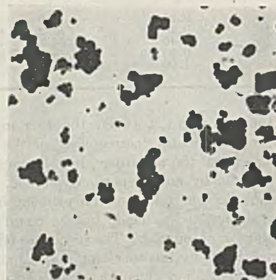
Figure 8. Electron Micrograph of Titanium Dioxide, \times 15,000
