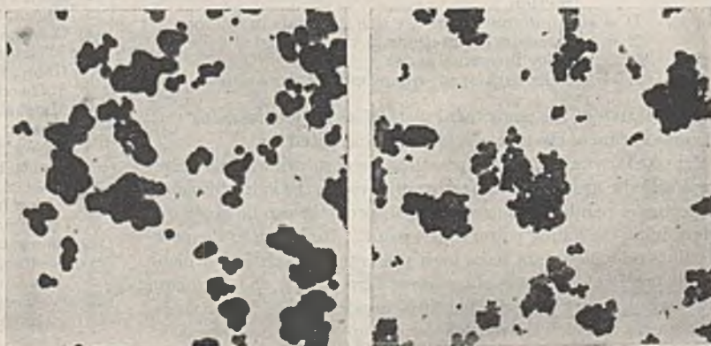
Figure 6. Electron Micrographs of Titanium Dioxide, ×15,000
