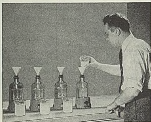
Any number of Fisher Filtrators can be assembled in series, for convenient operation.
