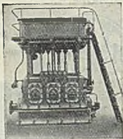
5-STAGE COMPRESSOR 400 Atm
