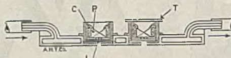
Cross-section of Nichols Refractometer, indicating water circulation within jacket. P, prisms; C, cement; L, engraved line; and T, cover glass
