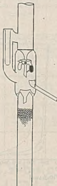
Figure 2. Reflux Controller and Top of Helices-Packed Column
