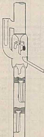
Figure 1. Reflux Controller and Top of Gauze Plate Column
