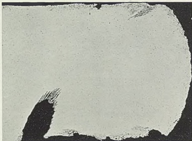
FIG. 5.— \frac{3}{16} -in. dia. 5% Magnesium Alloy Rivet after Accelerated Corrosion Test. \times 40 .
