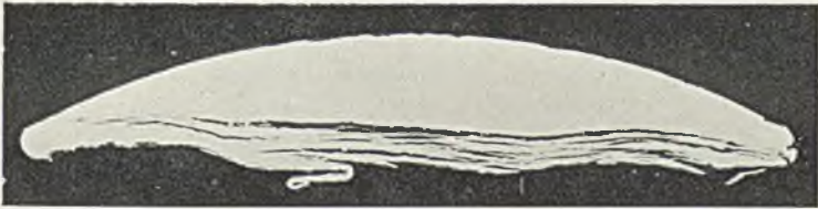
FIG. 3.—Foliation of 7% Magnesium Alloy Rivet Head. × 15.
