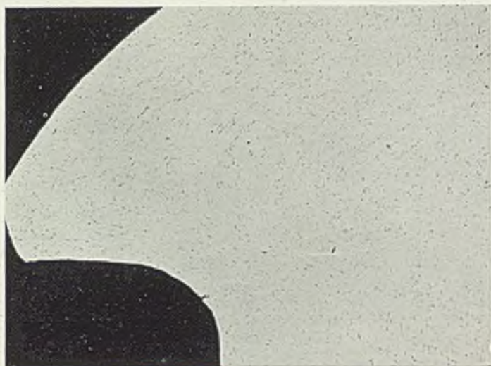
FIG. 6.—5% Magnesium Alloy Rivet As Received. Etched. \times 40 .
