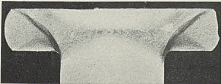
FIG. 4.— \frac{3}{8} -in. dia. 5% Magnesium Alloy Rivet, as received. Etched. × 10.
