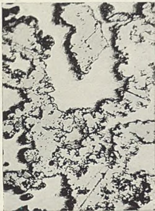
FIG. 4.—Aluminium-Thorium Compound Found in Residue from Melt of 5% Aluminium Alloy Treated with Thorium. \times 350 .
