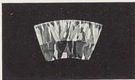
FIG. 8.—Macrostructure of Part of Cracked Ring Casting in 1% Silicon Alloy.
