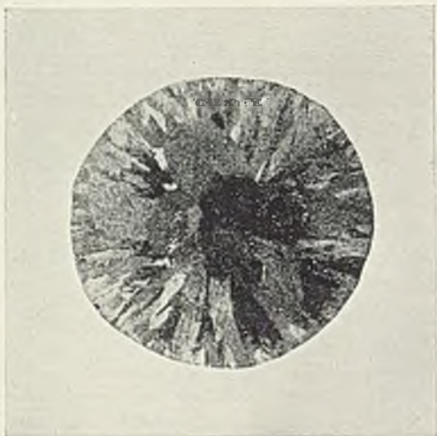
FIG. 3.—Cross-Section of D.T.D.-Type Sand-Cast Test Bar in 5% Aluminium Alloy Treated with Thorium. Macro-etched. \times 2 .
