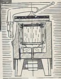
Diagrammatical representation illustrating the principles of the Vertical Forced Air Circulation Furnace.
