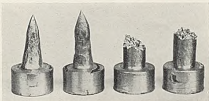
FIG. 7.—Super-Purity Aluminium Samples Tested at 498^{\circ} , 652^{\circ} , 656^{\circ} , and 659^{\circ} C., respectively. Natural size.
