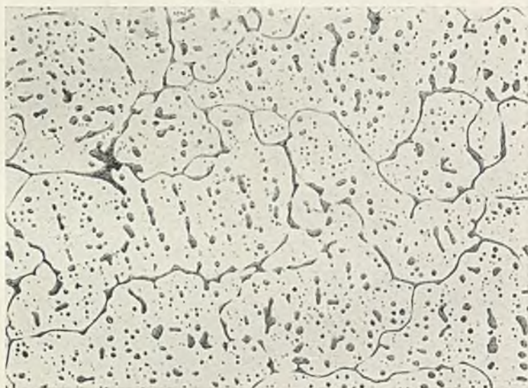
FIG. 13.—4%-Silicon Alloy Quenched from 580° C., Showing the Distribution of the Chilled Silicon-Rich Liquid. \times 75 .
