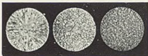
FIG. 12.—Microstructures of Chill-Cast Rods of 99.5% Aluminium (Columnar) and of 1% and 8% Silicon Alloys (Equi-Axed).
