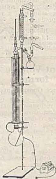
Fig. 2. The Towers Fractional Distillation Unit.
