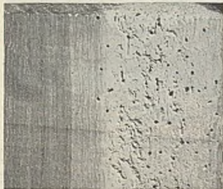
Fig. 2. Damage by Lyctus powder-post beetles in the sapwood of oak ( \frac{1}{2} nat. size).
