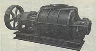
One of the many Holmes-Connersville Blowers supplied to Chemical Works. Capacity of machine illustrated, 120,000 cu. ft. per hour against a pressure of 3 lbs. per sq. inch. Speed 400 r.p.m deliver a positive, reliable and oil-free supply of Air economically and efficiently.
