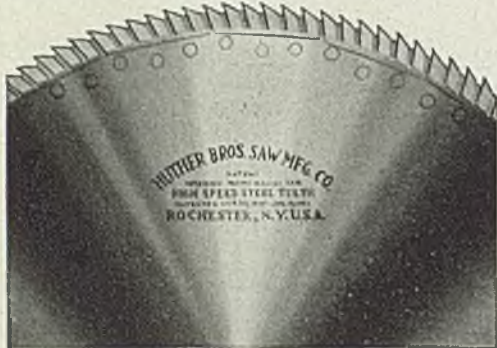
Segment with Firthite tips for Huther Bros. Patent Inserted Tooth Saw.
