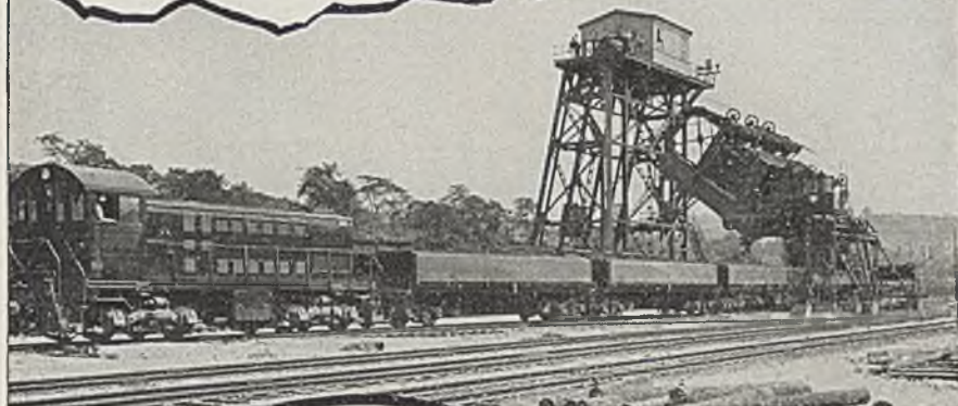
Ore being dumped into Rolling Trunnion Air Dump Cars, from standard railroad car dumper.
