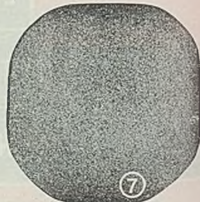
Fig. 7—Macroetch test specimen of typical ingot
