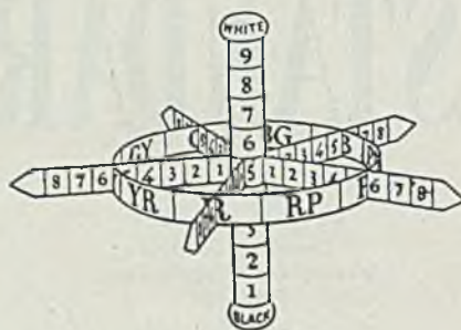
Fig. 2—Diagram showing hue, value, and chroma in their relation to one another. The circular band represents hues in their proper sequence. Upright center axis is the scale of value. Paths pointing outward from the center show steps of chroma increasing in strength as indicated by numerals
