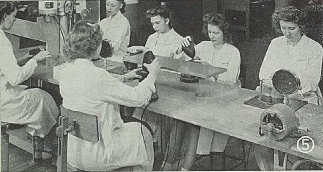
Fig. 5—Vacuuming and investing the flask. Six wax patterns are being invested in a flask 2½ in. in diameter and 2½ in. high. Eight to 10 girls can invest from 1500 to 2000 flasks per day
