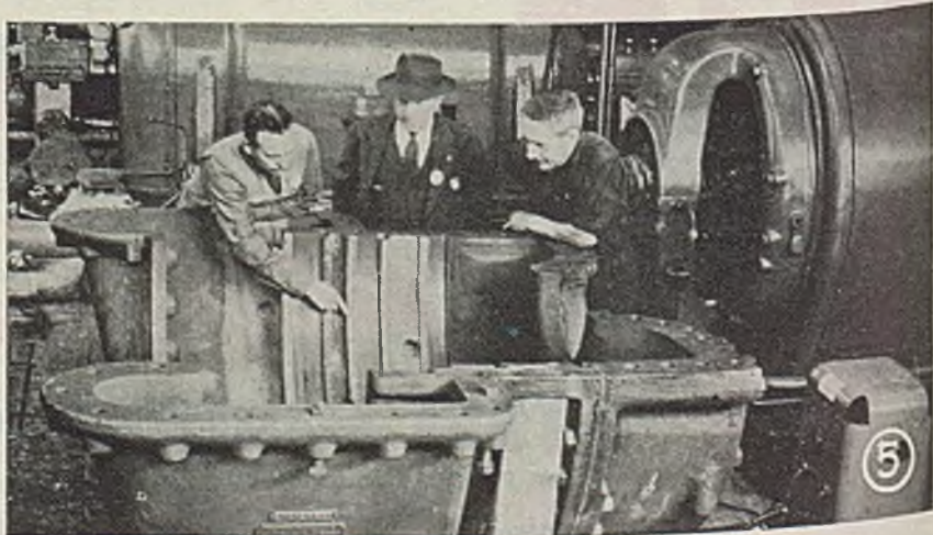
Fig. 1—Rim of turbine housing after last stage diaphragm was removed. Erosion was severe, averaging \frac{3}{8} -in. in depth
