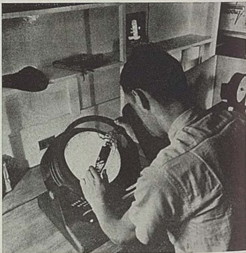
COLORS REVEAL STRAINS: Operator inspects an HF300 diathermy tube in the polariscope at the Brooklyn plant of the Amperex Electronic Corp. Electronic tubes are examined for strains in the glass after heat treating processes are completed. If strains are present, annealing removes them
