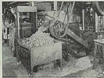
Receiving skid loads of material from blanking press for delivery to next process.
