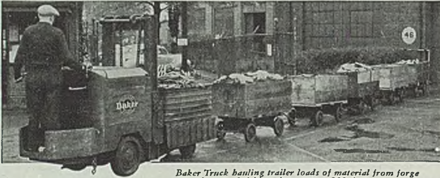
Baker Truck hauling trailer loads of material from forge shop to finishing department 300 feet away.
