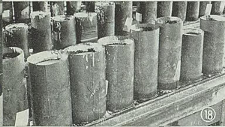
Fig. 18—After the mold has been filled with the investment, it is placed on a vibrator or “shaker table” to eliminate air and pack the material tightly. In about an hour, the investment has set and the fines risen to the top. Excess material above the top of the mold then is sawed off and the mold allowed to age for several hours. The steel plate is knocked off, exposing the mouth of the gate into which the metal will be poured later
