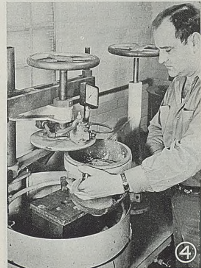
Fig. 4—Diemaker is preparing to pour the metal into the first half of the mold
