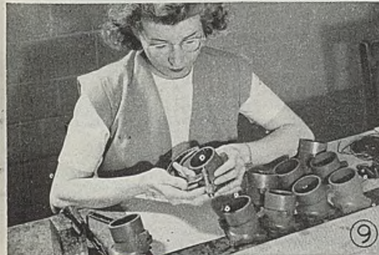
Fig. 9—This assembly line operator is checking the wax pattern for dimensional accuracy
