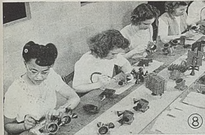
Fig. 8—In the assembly line of the wax department, operators inspect the patterns as they move by on a conveyor belt. The patterns then are assembled to gates and risers by "wax welding" and mounted on wax hubs molded especially for the purpose
