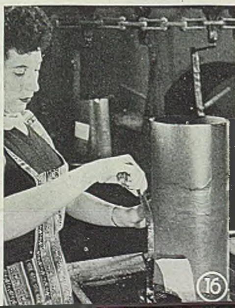
Fig. 17—The flask containing the wax assembly then is carried to the next department on an overhead hanger-conveyor where it is filled with a chemically-hardening investment material. This material, comprising tetraethyl silicate, crushed firebrick, silica sand and alcohol, is mixed on the floor above. The small mixer shown at the operator's right is filled as required by means of a chute
