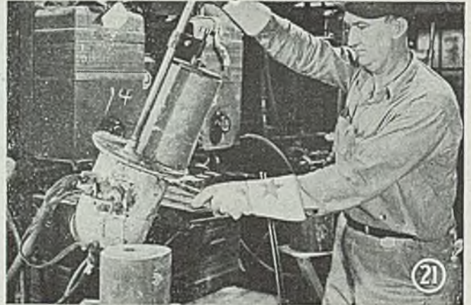
Fig. 21—Just enough metal in pig or “stick” form is melted down in this small indirect arc furnace to fill one mold. When the metal reaches the correct temperature, as checked by an optical pyrometer to insure proper grain size and other desired metallurgical properties, the hot, baked mold is inverted directly over the pouring spout of the furnace. After the mold is clamped in place, the metal is poured by inverting the entire furnace and turning on about 3-lb air pressure from a line connected to the furnace. Air pressure makes possible casting of dense structures and the filling-in of thin edges
