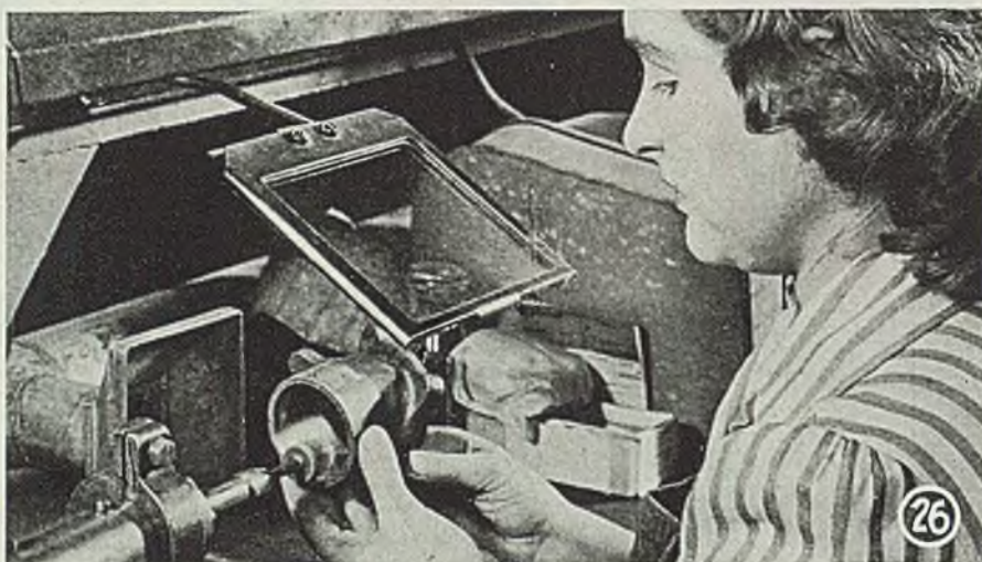
Fig. 26—Inside areas are touched up as needed with a small internal grinder
