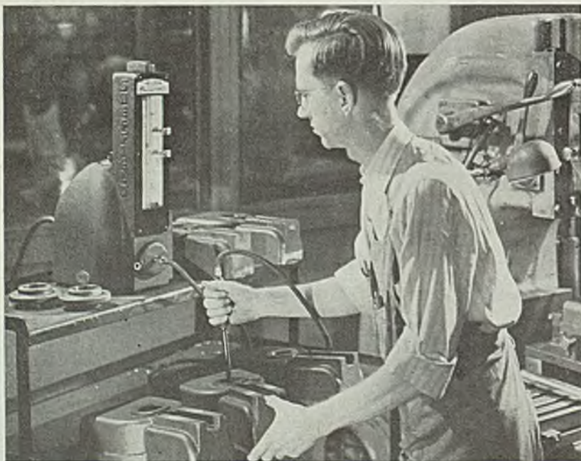
PRODUCTION-LINE CHECK: Use of the Precisionaire gaging unit, made by Sheffield Corp., Dayton, O., at a vertical boring mill is said to increase production, reducing scrap to less than 2 per cent. In above operation, checking column hole of a visual gage base casting, gaging unit holds tolerances to 0.0005 in.
