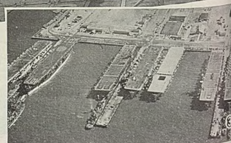
Fig. 3—These escort carriers at Norfolk, Va., are being subjected to preservation methods. Note carrier third from right already has complete coat of haze gray paint, developed by the Navy
