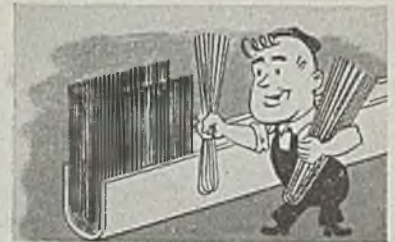
2 Then, filler material of the kind and length to do the job best is "hairpinned" and inserted, ends up, in the channel.
