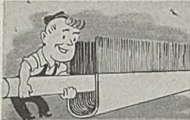
3 Next, a plated steel wire is laid along the channel on top of the filler material to anchor it permanently in position.
