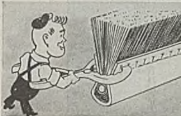
4 Finally, the sides of the metal strip are clinched under heavy pressure so that the bristles can never fall out.
